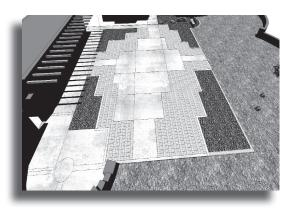
In early March, the Visitor Center closed for the first in a series of upgrades. These include taking out the asphalt driveway an installing permeable concrete pavers for better drainage, renovating the patio and putting in a shade structure, and making repairs to the floor inside the building.
